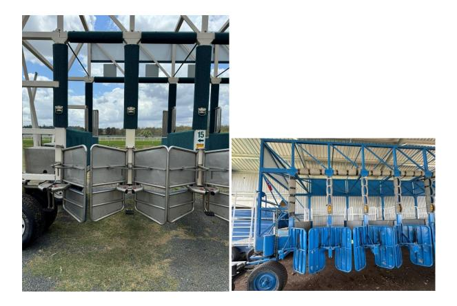
Ripped and torn padding must be repaired:
