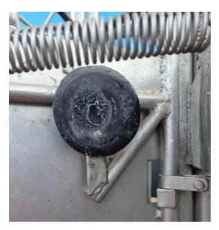
Damaged gates should be straighted and adjusted to ensure they fully close, the following are examples of gates that are not correctly aligned.
